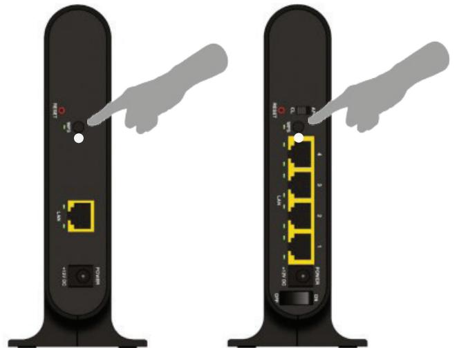
8. Return to the set top box and press the OK button located on this box (not on the remote control). If your set top box does not have an OK button, press the Power button instead.
